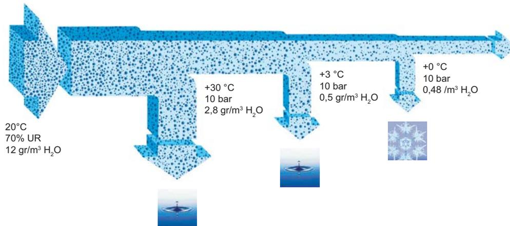
The cooling process does not allow the temperature to fall below 0°C (solidification of water). However, specific applications or particular ambient conditions require dew point temperatures of below 0°C.
