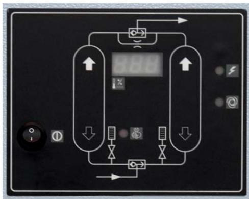
The electronic Pressure Dew Point control (CD) extends the drying phase of the dryer's cycle. It is done by measuring PDP of compressed air on the dryer outlet and only switching the columns when desiccant in the active tower is saturated. The regeneration part of the cycle stays fixed.
