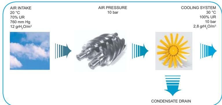
Compressed air is cooled at 30°C and condensed water vapour is separated, while 2.8 gr of water for every Nm<sup>3</sup> of air that condense can remain in the air (compressed at 10 bar as in the example) in vapour form.
