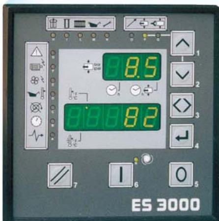
**Control panel** with state-of-the-art control system, microprocessor diagnostics and alphanumeric display for safe, efficient machine management. All data displayed in standardized symbols
